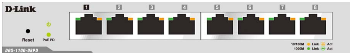
Figure 1.5 –LED Indicators on DGS-1100-08PD
